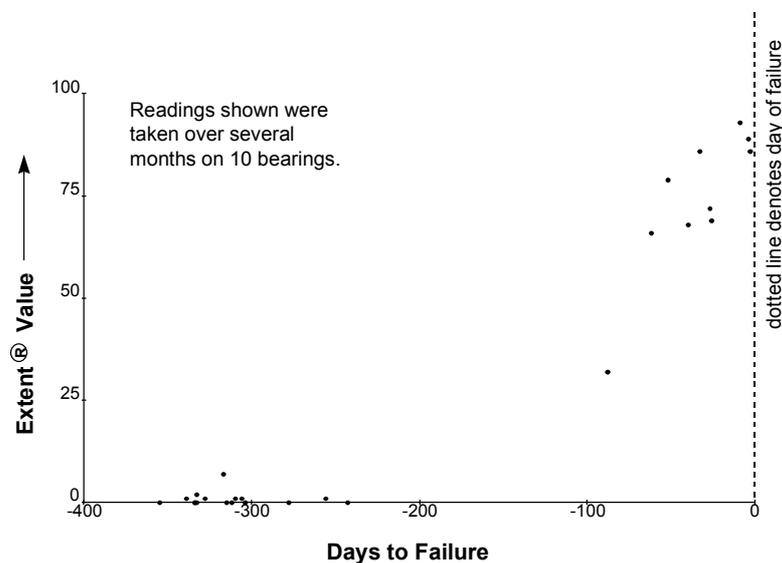
Figure 2 : Sensitivity of ' Extent® ' to proximity of failure in turntable bearings.
