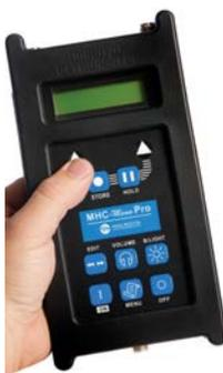
The Memo Pro is able to monitor a near unlimited number of machines on a periodic basis. In addition to storing Standard and Super Slo modes within its walk around routes, the Memo Pro can also store manually input values from any other device (e.g. a pressure gauge, kVA meter etc.). The Memo Pro can hold up to 6 routes at a time, each having up to 435 measurement points within a Site, Area, Machine & Point hierarchy.
