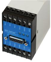
The MHC-Point/Slo is capable of monitoring virtually any rotating piece of equipment rotating at speeds from 60 rpm down to 0.25 rpm without knowing anything about the detailed design of the machinery. This capability to monitor very slow rotational speeds in a unique attribute of AE technology complimenting & extending the range of any existing limitation monitoring programme.
