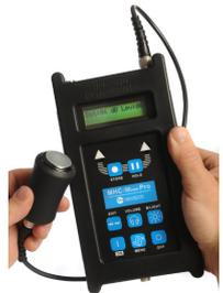
At the conclusion of this trial the workshop based craftsmen were equipped with an MHC instrument which they now use on a day to day basis. Not only was the MHC found to be equally as effective as the FFT based high frequency demodulation instrument in detecting faults but it had the additional benefits :
