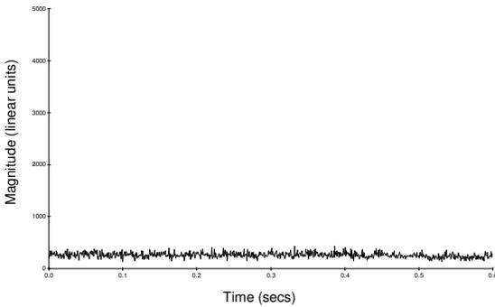
Figure 2(a) – Dynamic envelope signal from a roller bearing in good condition.
